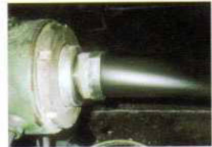
Ecologix's EPDM tubing extrusion and plastic injection
